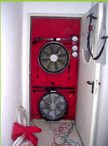
picture 5.1 — installing a Blower-Door; Source: BlowerDoor GmbH
